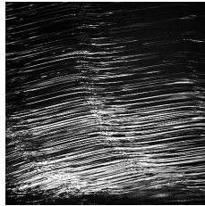
Wiping of a fingerprint with non-decontaminated cleaning wiper, mesh density 400 = no residues
