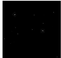
After imprint of decontaminated knitted wiper (hardly any particles)
